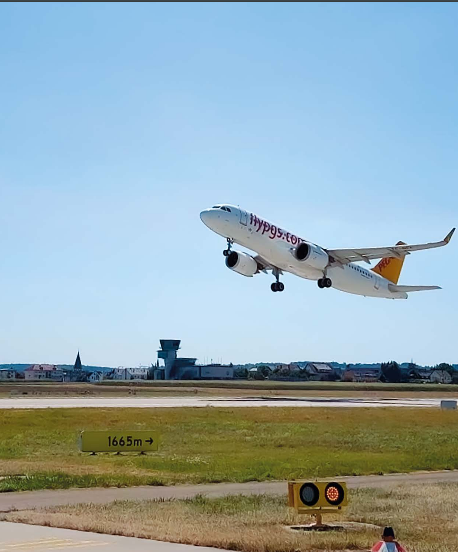
Runway Guard Lights in EDDS, Rollhalt E, RWY 25. Foto: Florian Huber
